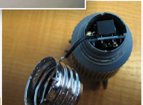
Figure 5 The power-management PCB fits into the base of the bulb.
