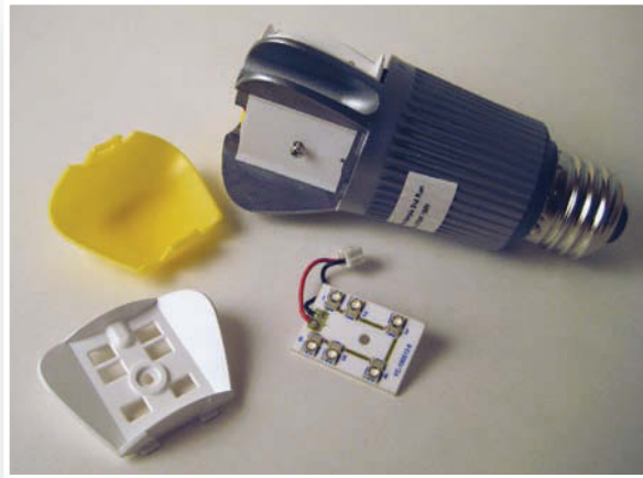
Figure 4 The LEDs mount vertically on the bulb's heat sink.
