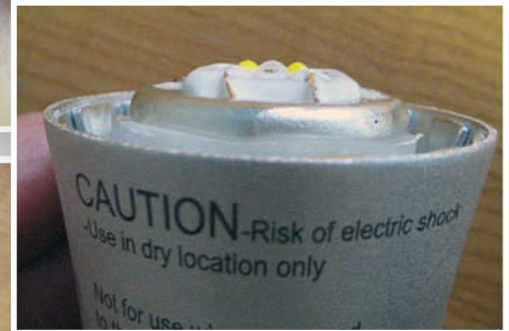
Figure 11 The LED's array (below) is slightly elevated. As a result, it projects down more than it would if you aligned it with the edge of the LED's heat-sink base.
