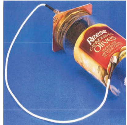
Figure 2 A plate of copper-clad PCB material stiffens the metal cap of the olive jar. The transducer mounts inside the jar, and an SMA header allows a coaxial cable to connect to the assembly.
