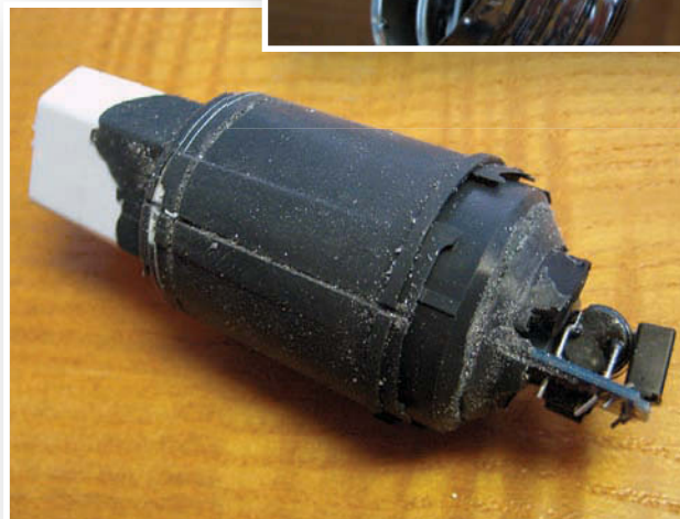
Figure 6 A rubbery potting compound encapsulates the power-management circuitry.
